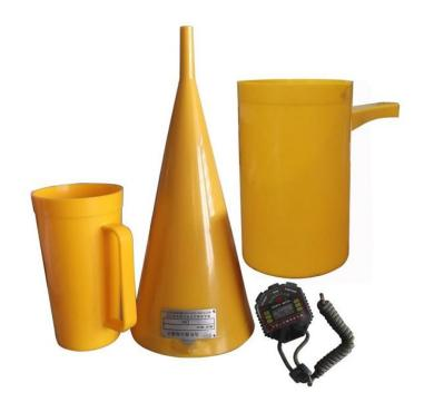
漏斗粘度计 Funnel Viscometer
